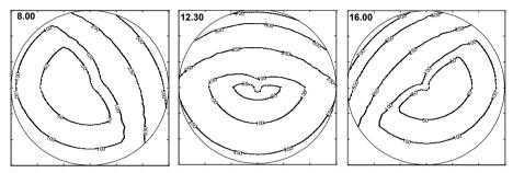
Figure 3. Cross-sectional light profile ( $W m^{-2}$ ) inside a single horizontal tube in the Netherlands at 8:00, 12:30 and 16:00 hours on a clear sky day (30 June 2009) as seen from south. Reactor is oriented on north-south line, tube diameter is 0.06 m and characteristics of the algae species *P*. tricornutum have been used with a biomass concentration of 1 kg m<sup>-3</sup>.
