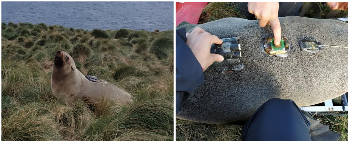
Fig 2: Photographs of an Australian fur seal equipped with data loggers (left) and of a video data logger, dive behaviour data logger, GPS data logger and VHF transmitter, glued to the dorsal fur (right).
