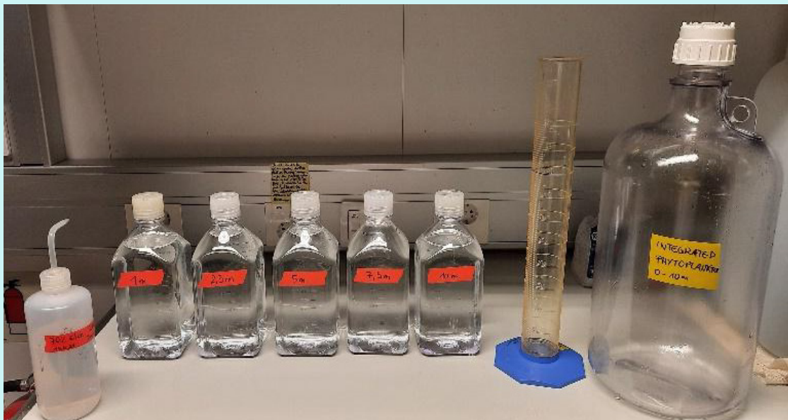
Figure 1. Water samples from 5 different depths (1 m, 2.5 m, 5 m, 7.5 m and 10 m) and required equipment to prepare the integrated sample (0-10 m). Photo: Jacqueline Jerney.
