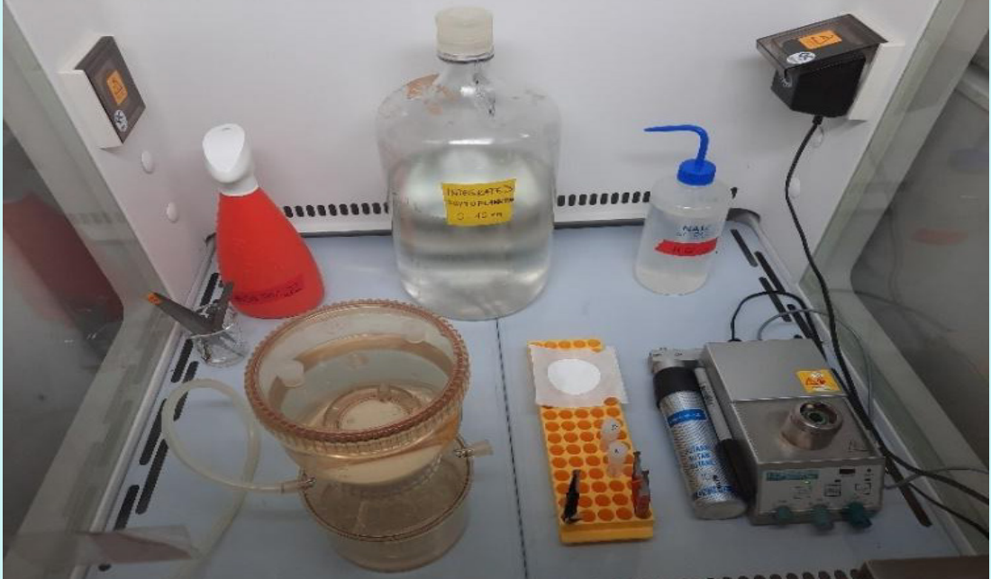
Figure 2. Filtration set-up in the laminar flow hood onboard the research vessel. If there is sufficient space next to the laminar flow hood, the Bunsen burner should be placed outside of the laminar. Photo: Jacqueline Jerney.
