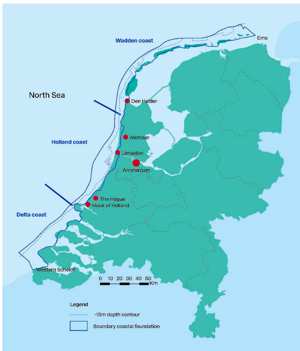
Fig. 1. Overview of the coastal zone of the Netherlands. Indicated are the boundaries of the coastal foundation, the -15m contour, the Delta- Holland- and Wadden coasts, major coastal cities and the Ems and Western Scheldt estuaries.
