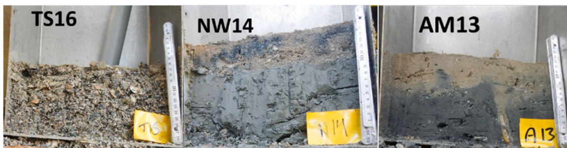
Fig. 18. Rectangular box cores collected in 2018 with the side detached. Box core TS16 (NW corner Terschelling area; left panel) shows a coarse-grained shell layer. Box core NW14 (Noordwijk area; middle panel) shows a sand layer overlying a stiff blue-grey clay. Box core AM13 (delta front, Ameland Inlet area; right panel) shows a layer of brown, oxygenated sand on top of dark grey sand that is poor in oxygen. Directly left of the yellow label sits a razor clam that has dug itself in, probably in reaction to the penetration of the corer into the seabed and its subsequent extraction. Scale in cm.
