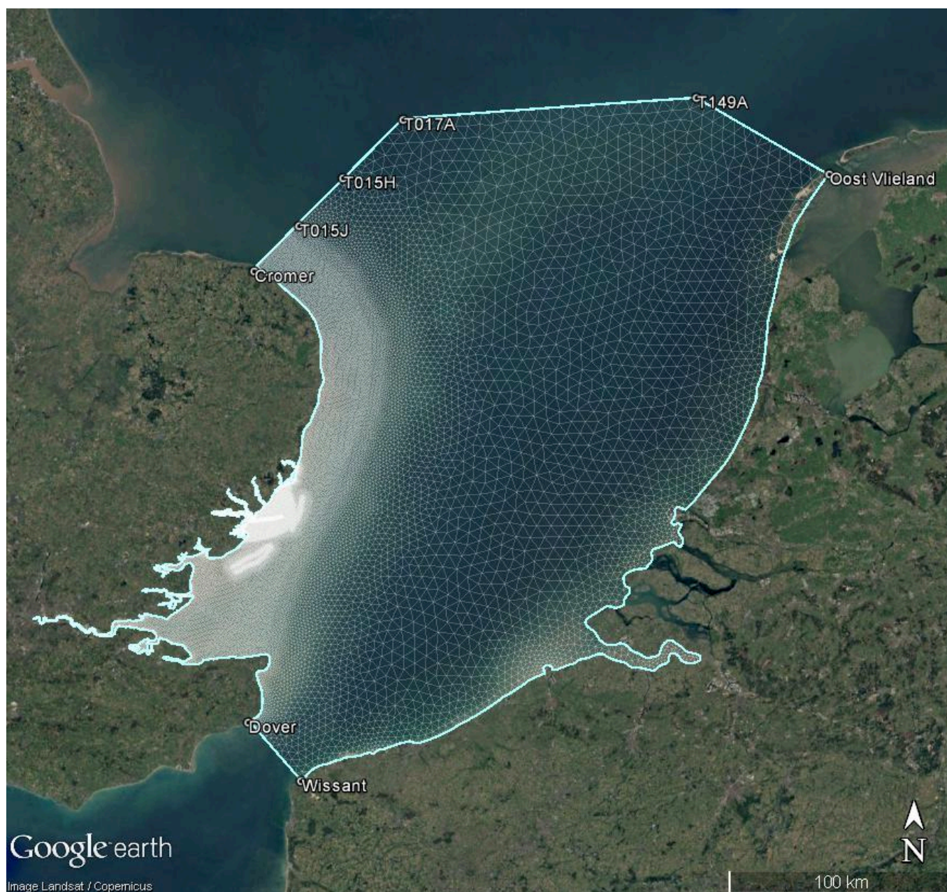
Figure 5. Model domain and mesh, showing locations of Admiralty tide gauge stations used
