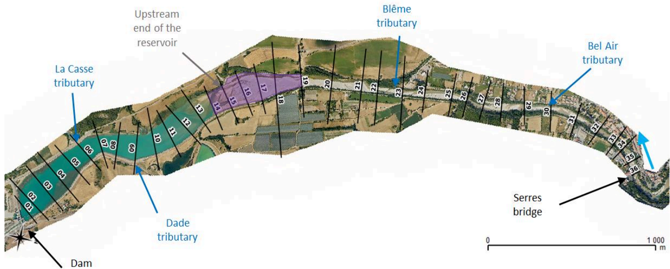
Figure 10: Presentation of the study site. The black lines indicate the cross-section locations of the bathymetric surveys.
