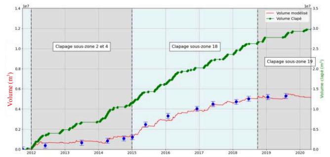
Figure 15. Calibration result for in-place volume – Model in red line, dumped volume in green line and in-place volume data in blue dots
