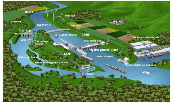
Figure 2. Typical CNR reservoir
