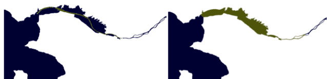
Figure 8. Initial fluid mud conditions (mud: green, no mud: blue): liquid fluid mud on the left, stricto-sensus and consolidated fluid mud on the right
