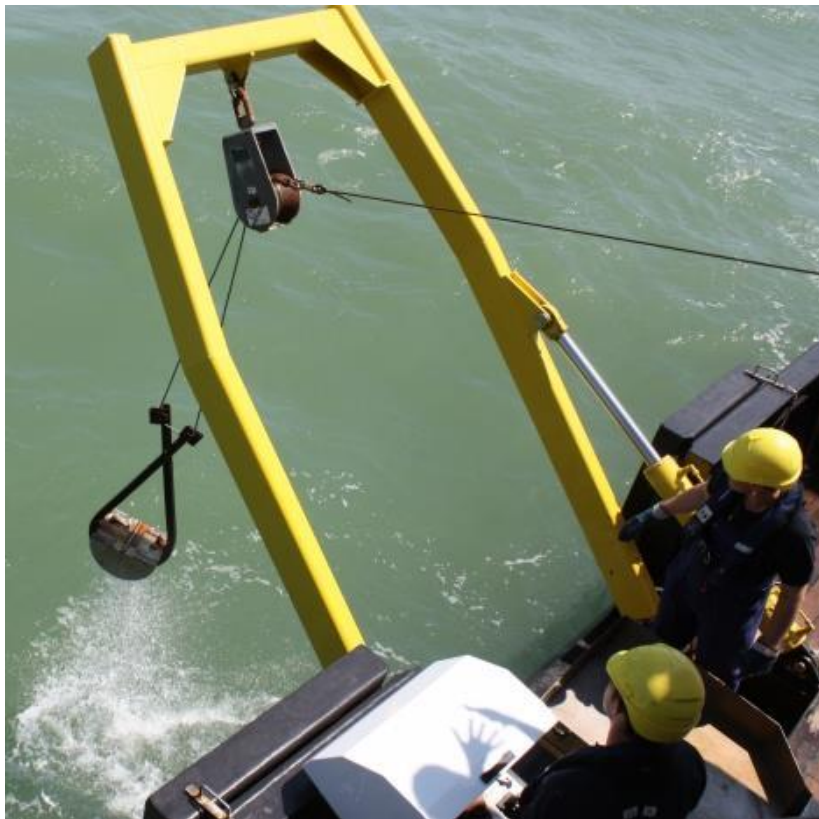
Figure 4.- Image of a Van Veen grab used to collect sediment samples. Source: Flanders Marine Institute (VLIZ) - Mertens, Tina).
