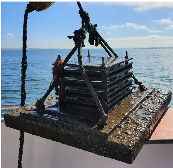
Figure 1: An ARMS, including the concrete paver.
