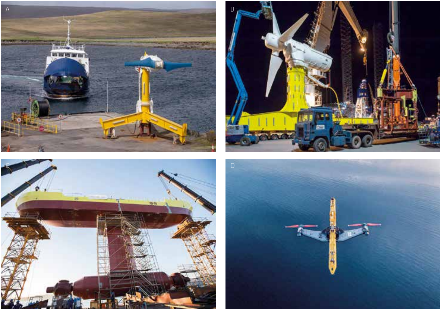
Figure 2.10 MW-size tidal turbine prototypes. A: Shetland Tidal Array device; B: MeyGen Array device; C: Assembling the main structure of the Magallanes Renovables device; D: Orbital Marine Power device.
