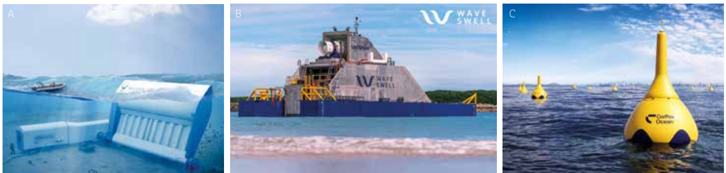
Figure 2.8 Wave energy converter prototypes. A: AW-Energy's WaveRoller; B: Wave Swell Energy's UniWave device; C: An artist's impression of a CorPower C4 wave farm.
