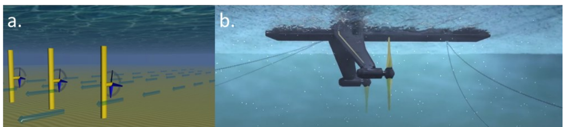
Figure 1-4 Illustration of different forms of tidal energy extraction technologies: a. seabed mounted turbines (source: Aquaret, 2012) b. floating platform (source: Orbital Marine Power Ltd)
