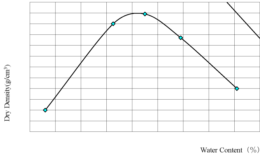
Figure 30 Relationship between Optimum Water Content and Dry Density
