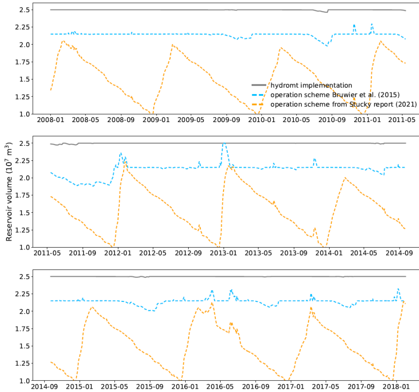
Figure C-6: Simulated reservoir volume for the Eupen reservoir for the period 2008 until 2018. The grey line indicates the simulations with the original HydroMT derivation, the blue dashed line indicates the simulations of step 1 and the orange dashed line indicates the simulations of step 2.
