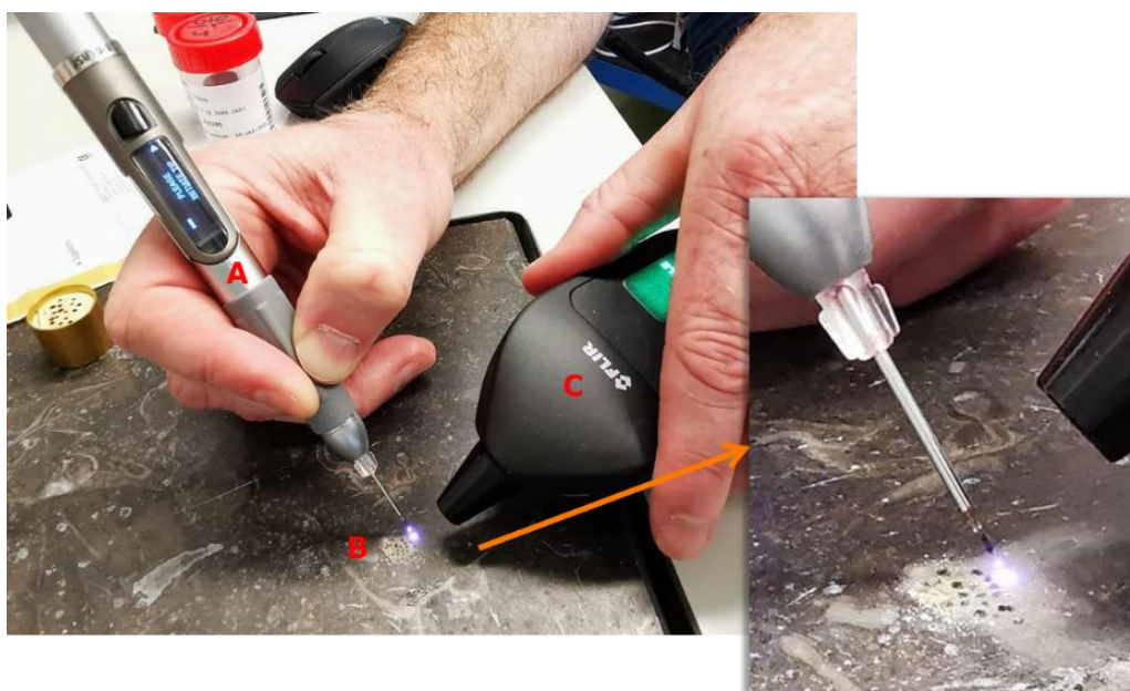
Figure 4. Overview of the experiment to identify a white powder left next to an analytical balance, A: Portable laser, B: white powder, C: Heated sampling probe.
