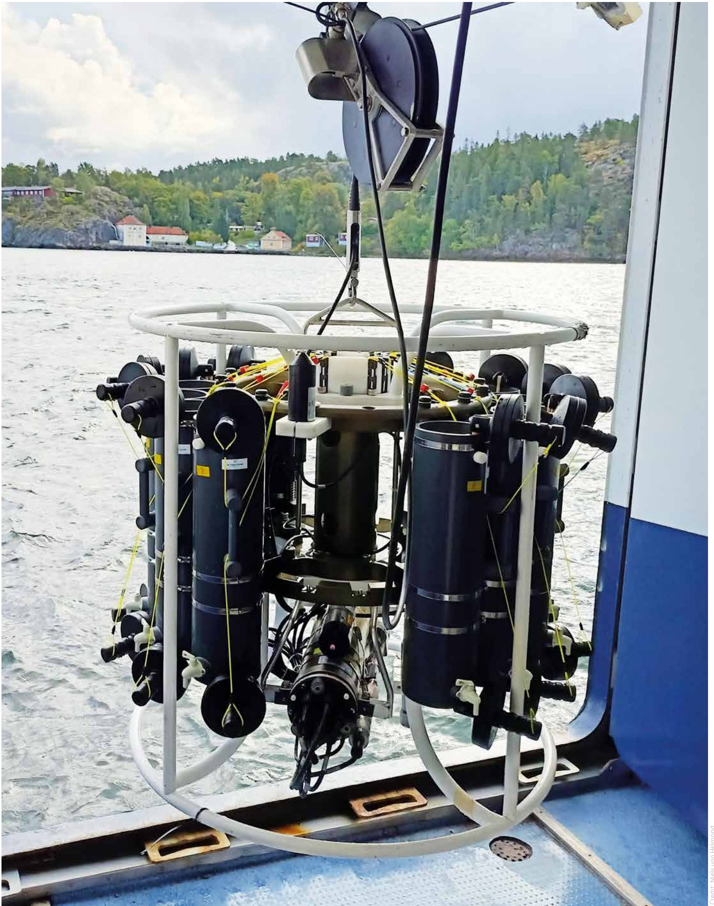
Figure 5.2 A Conductivity-Temperature-Depth (CTD) device. The combination of CTDs with dissolved oxygen sensors and Niskin bottle collections facilitates the continuous measurement of oxygen in the water column.
