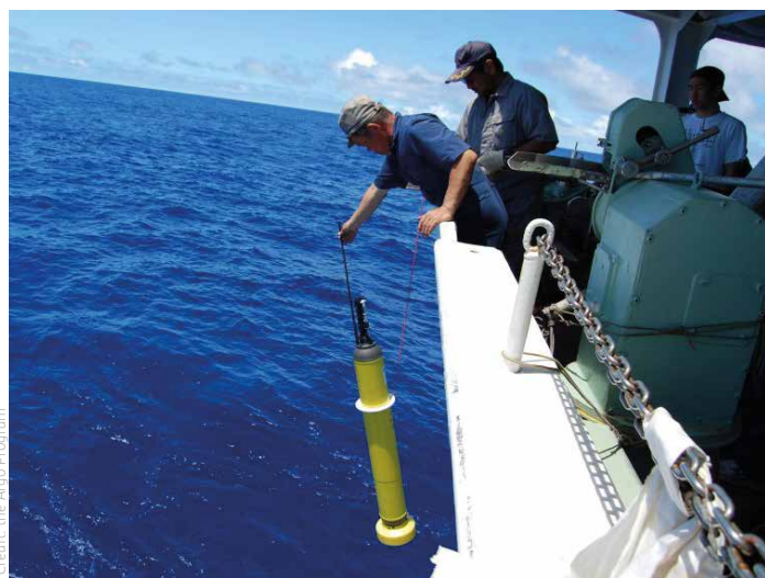
Figure 5.3 Left: An Argo float being deployed. Right: An Argo float with an oxygen sensor.
