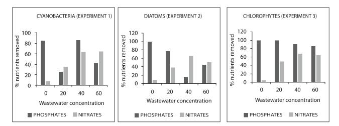
Figure 3. The percentage of nutrients (PO4<sup>3-</sup> and NO4<sup>-</sup>) removed from the wastewater cultures.
