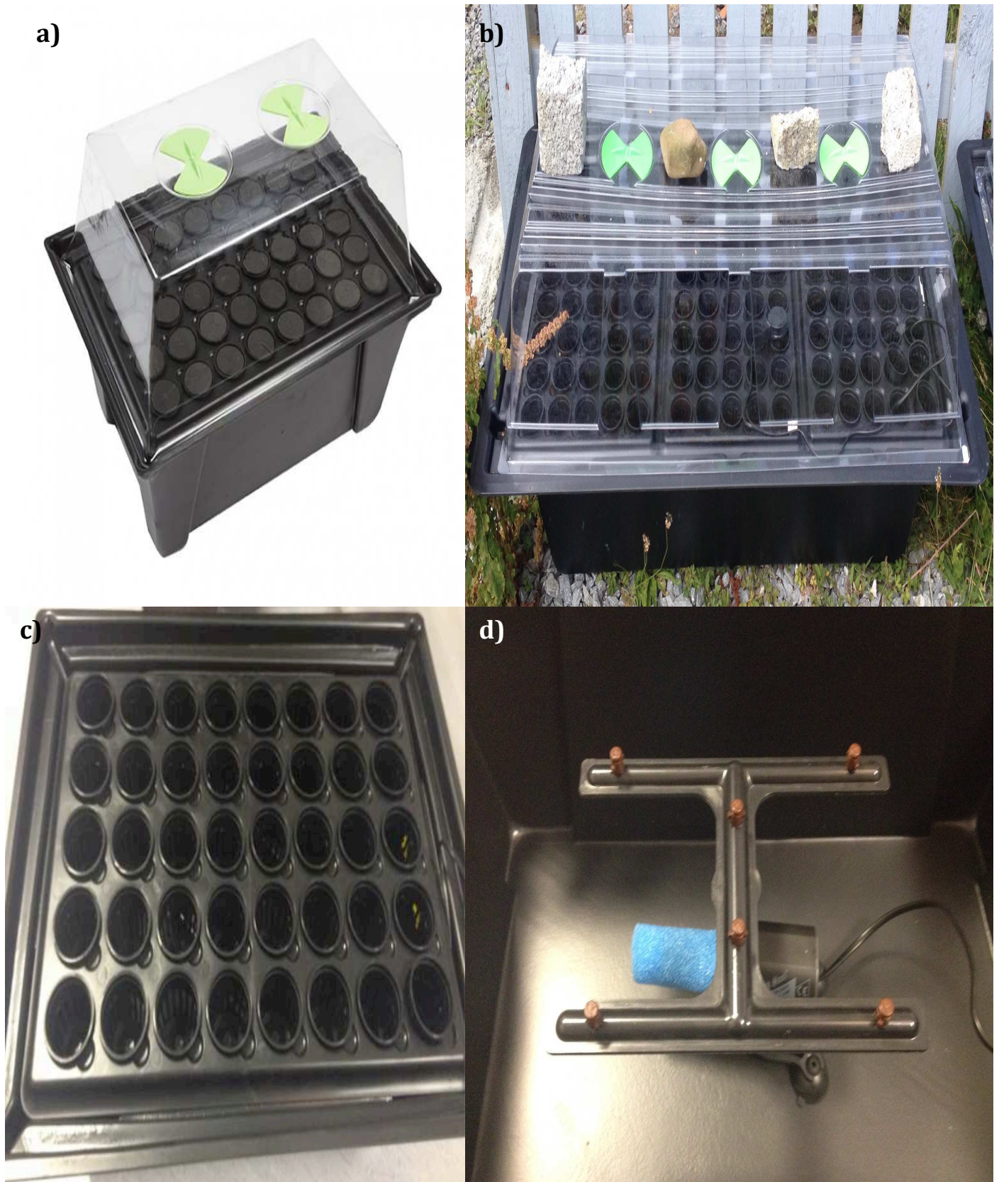
Figure 15: Example of a) 40 slot aeroponic propagator (dimensions: 60x50x40cm); b) 120 slot aeroponic propagator (dimensions: 115x64.5x46cm) c) 40 slot top tray; and d) the spray-bar in the reservoir below
