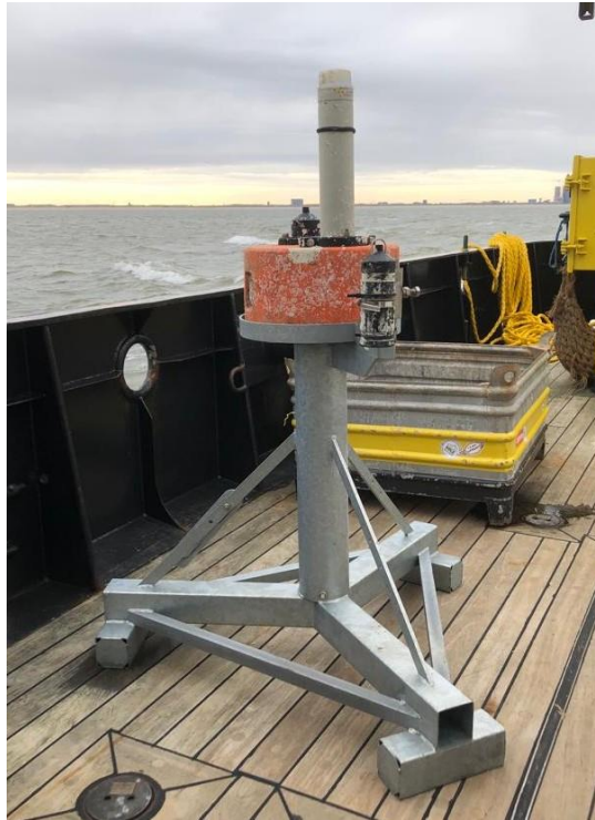
Figure 5.1. Multi-use platform of the Belgian passive acoustic network (BPAN) equipped with a C-POD and receiver.
