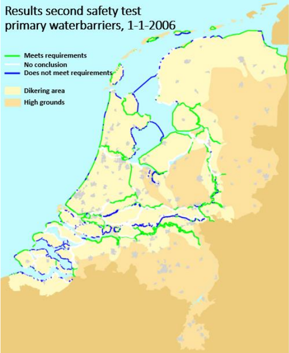
Figure 9 shows the results of safety test that has been conducted in 2006. This figure indicates that a lot of dikes within the delta area already don't meet the current requirements regarding flood risks. This does not mean that the dikes are not safe, yet probability of flooding or failure is higher than the national norms.
