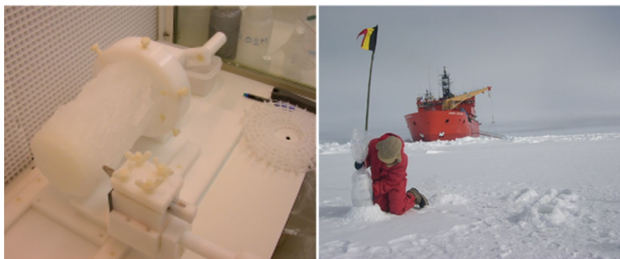
Fig. 1 Photographs of (left) ice-core cutting process and (right) sample placement for the in situ incubation. 1-cm-thick slices of sea-ice cores were cut using titanium chisels and blades under a class 100 laminar flow hood; bottom ice slices were transferred into acid-
