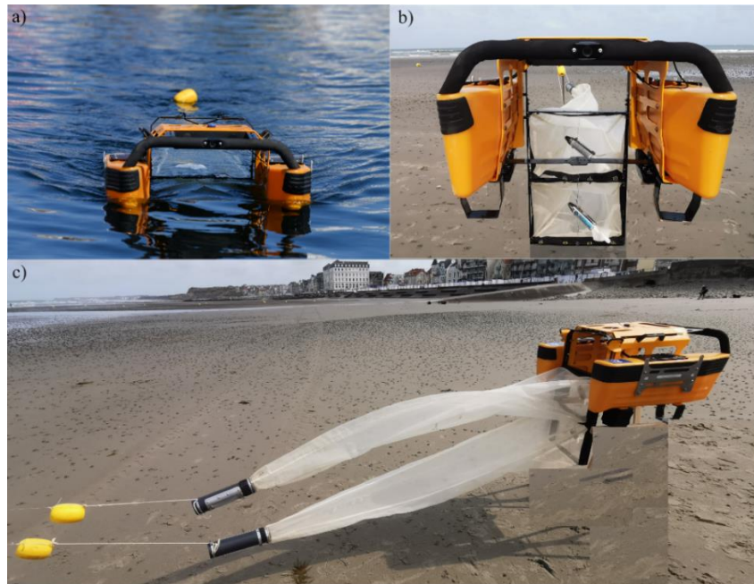
Figure 9: Aquatic drone a) and the removable metal frame b) designed with two nets levels (c)
