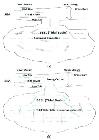
**Figure 1.** Tidal river management (TRM) mechanism in the Hari–Teka–Bhadra basin of the GBM delta. (a) Land reclamation due to sediment deposition in the tidal basin during high tide. (b) Strong
