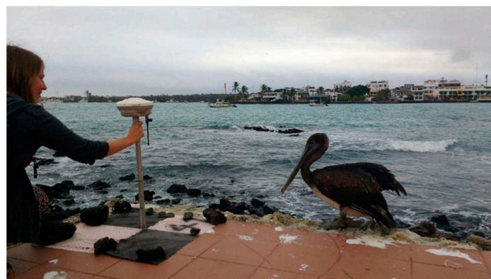
Figure 2. GCP measurement with Trimble 8 on a target sheet.
