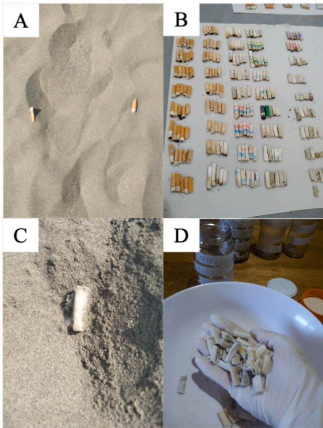
Fig. 3. CB and CBF samples in beach sand. A) Cigarette butts in beach sand, B) Method for quantifying cigarette butts (CB) in a laboratory, C) Fibers from cigarette butts (CBF) in beach sand, and D) Example of cigarette butt fiber (CBF) quantification in the laboratory.
