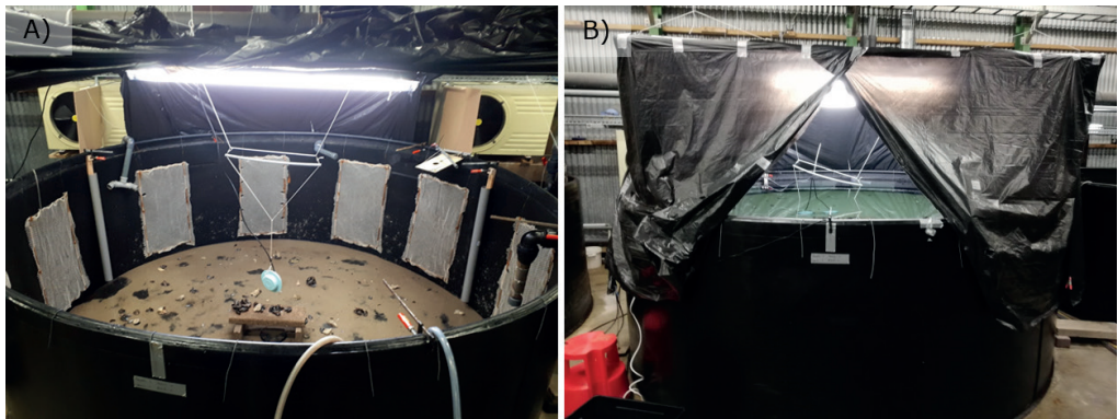
Fig. 1: Pictures of a cylindrical experimental tank. (a) The tank before being filled with water, but with sand on the bottom and patches of mussels, oysters, and some rocks for shelter. Also visible are the frame holding the TL light bars and underwater speaker and the white netting to increase the visibility of the fish and the PVC pipes to release the crabs. (b) The same tank now filled with water and covered with black plastic sheet.
