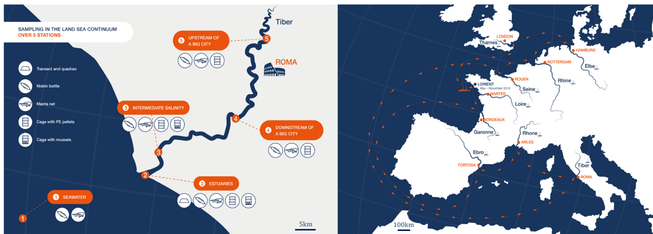
Fig. 1 Sampling strategy in the land-sea continuum. Left: Example of sampling strategies in the Tiber River (Italy) along the salinity gradient from the sea (station 1), the outer estuary (station 2), intermediate salinity (station 3) to downstream (station 4), and upstream (station 5) of the first heavily populated city (Rome). Samples were
