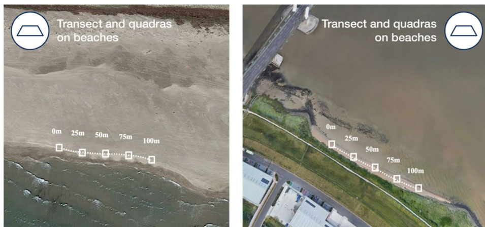
Fig. 3 Sketch of the sampling protocol for macro-, meso-, and microplastics on beaches (left) and river bank (right). Squares are the five quadrats of 0.50 m length sides ( 0.25 \text{ m}^2 ) along the high tide (dotted line)
