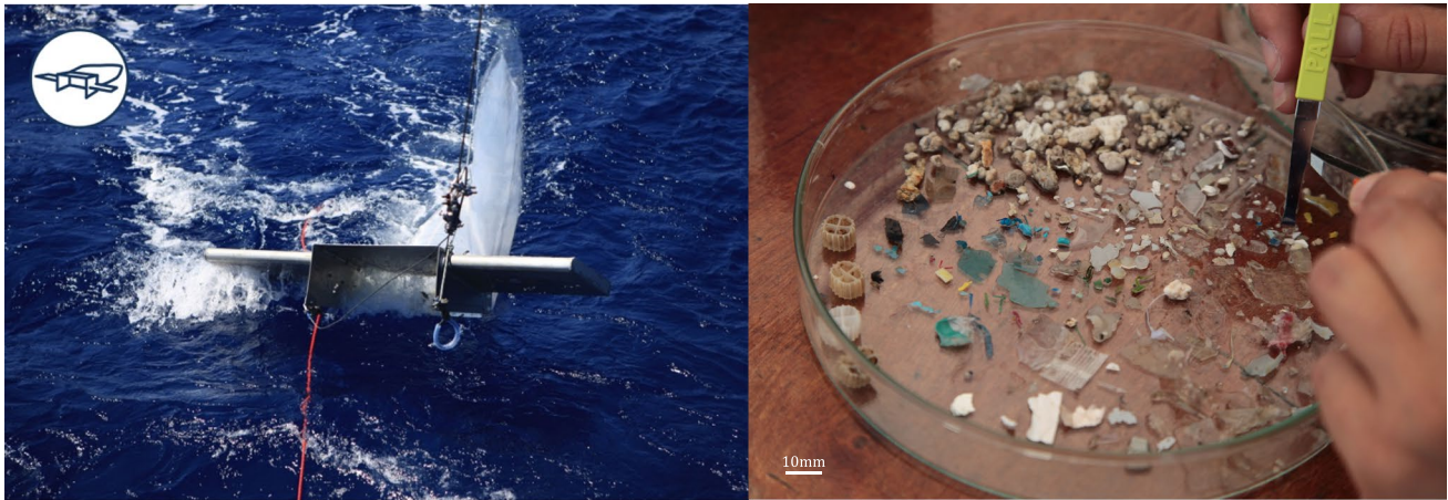
Fig. 2 Photographs of the 330- \mu\text{m} mesh size manta trawl (left) and the following microplastic sorting with sterilized forceps (right) (credit to Noélie Pansiot, Tara Ocean Foundation)
