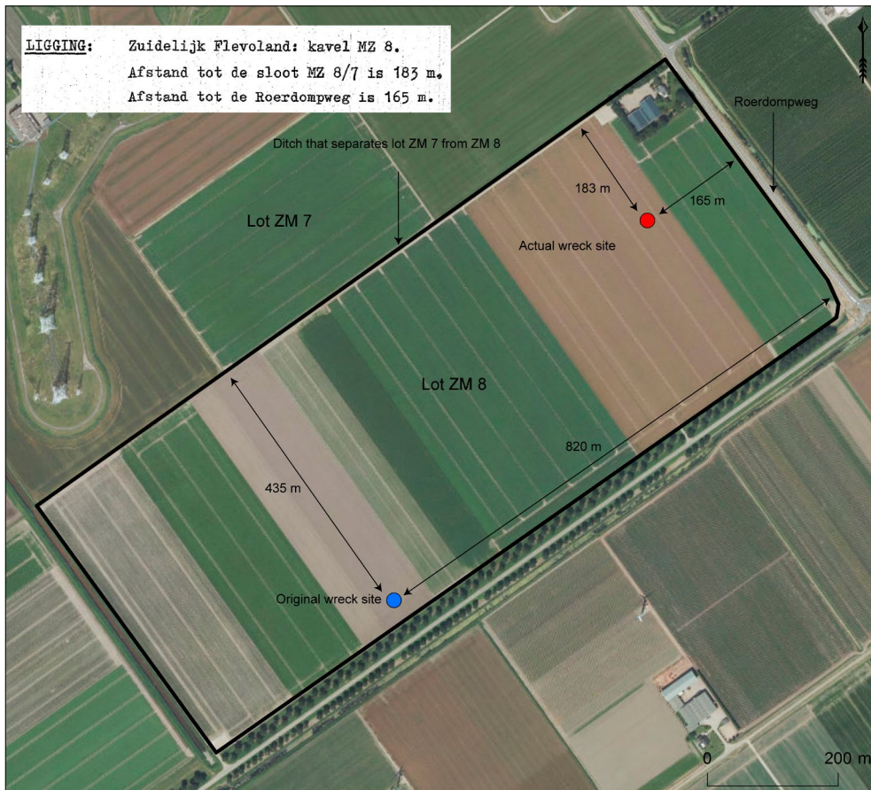
Figure 5.6. This figure shows the actual wreck site of shipwreck ZM 8 (red dot) and its recorded location (blue dot). The use of random coordinates, while an accurate wreck site description was available, caused a deviation of 700 m.
