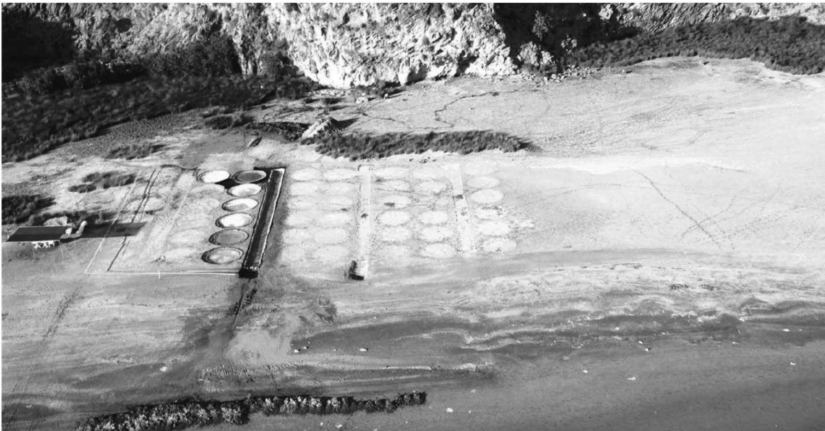
Figure 33 Salina of Caunus (Turkey) depicting all 48 circular salt pans arranged in eight lines of six pans separated by four large rectangular canals (Atik, 2008)
