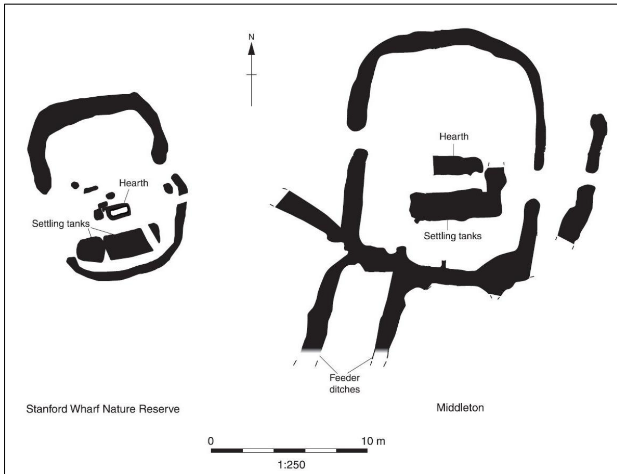
Figure 35 Working areas of the late Roman salt production sites at Stanford Wharf Nature Reserve (GB) and at Middleton (GB) showing the feeder ditches supply the salt water, the ditches defining the working area, the settling tanks and the hearth infrastructure (Biddulph et al., 2012, 160, figure 166.157).
