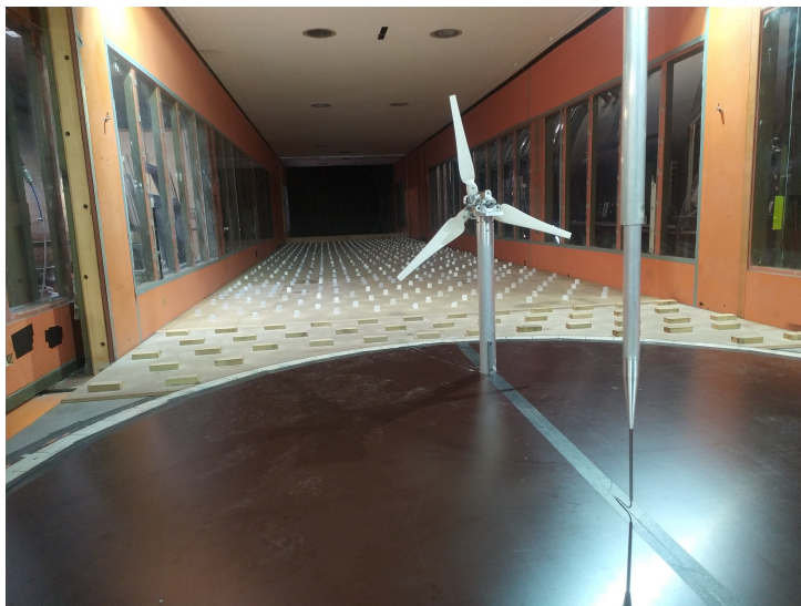
(a) Wind turbine and hot wire setup in the L1-B test section
