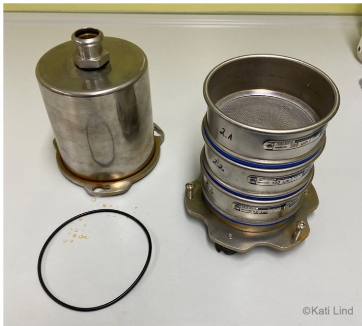
Figure 3: Inner container with three Retsch sieves
