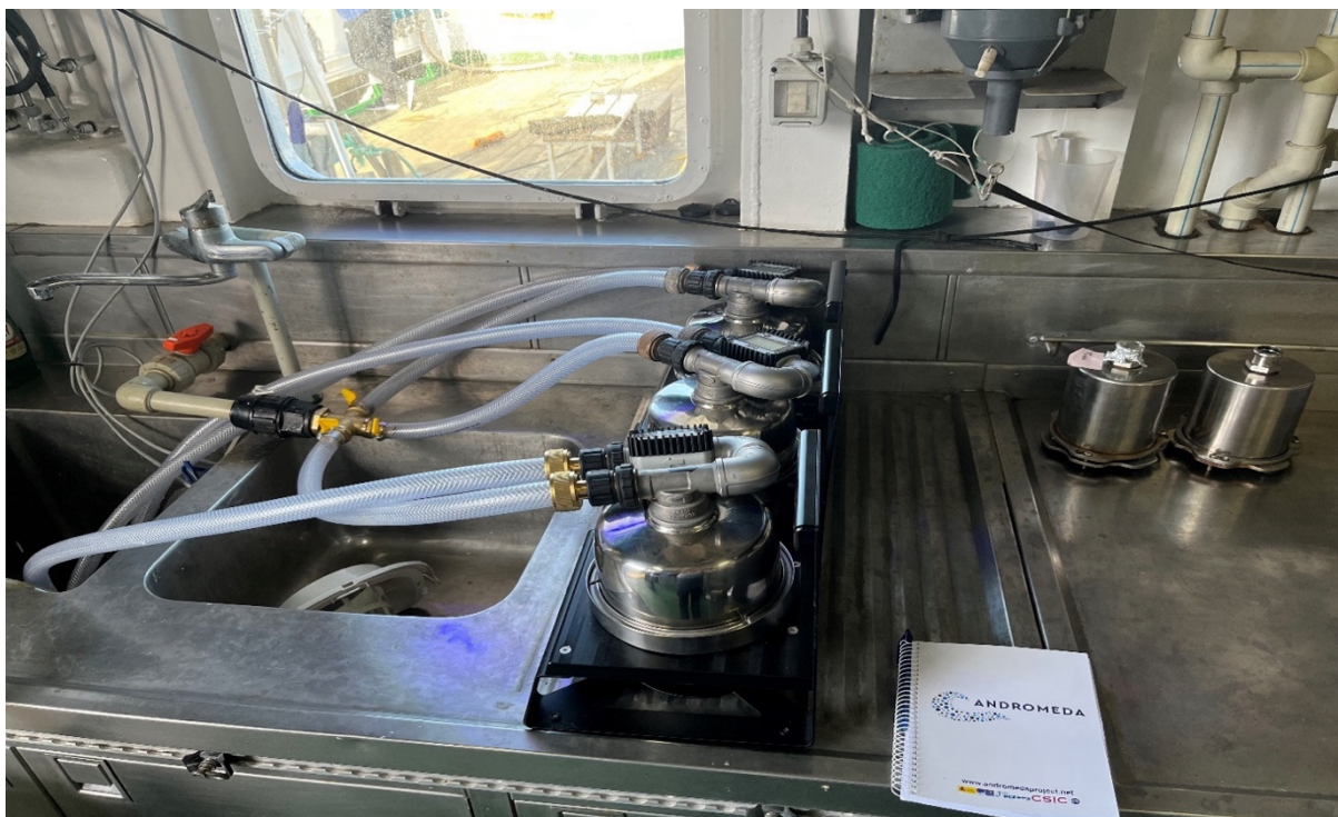
Figure 2: Microplastic sampling device outer container with black thumbscrew
