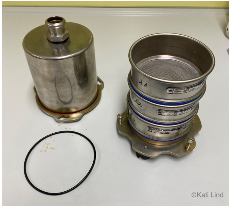
Figure 3: Inner container with three Retsch sieves
