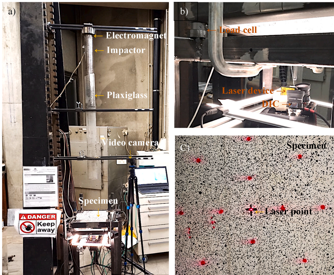
Fig. 2. a) Impact setup with 10 kg impactor released at the height of 1 m above the centre of a specimen, b) Location of DIC, Laser device and load cell, c) Laser pointing at the centre of the specimen.
