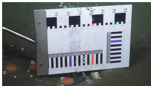
Fig. 25. A scale-bar board was used to roughly examine the estimated bubble sizes and rising velocity. Picture taken by ROV SuBastian, Schmidt Ocean Institute.
