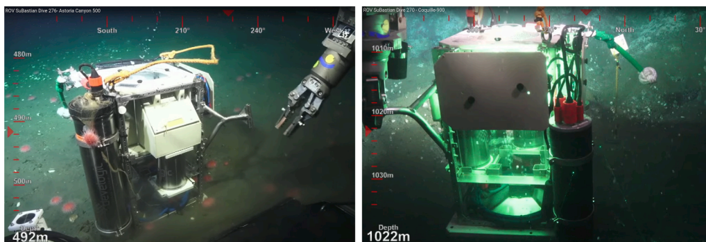
Fig. 2. Instrument deployed by a remotely operated vehicle (ROV) in 500 m and 1 km water depth in the Pacific Ocean offshore Oregon during Falkor cruise FK190612 'Observing Seafloor Methane Seeps at the Edge of Hydrate Stability' (see also https://youtu.be/fixiD75qmQFU for a recording of the entire live stream captured by ROV SuBastian, Schmidt Ocean Institute). The instrument is positioned on the seafloor over a seep spot where methane bubbles escape; bubbles rise through the instrument and are photographed by a wide baseline stereo camera setup at high frame rates for photogrammetric characterization of size, shape, rise
