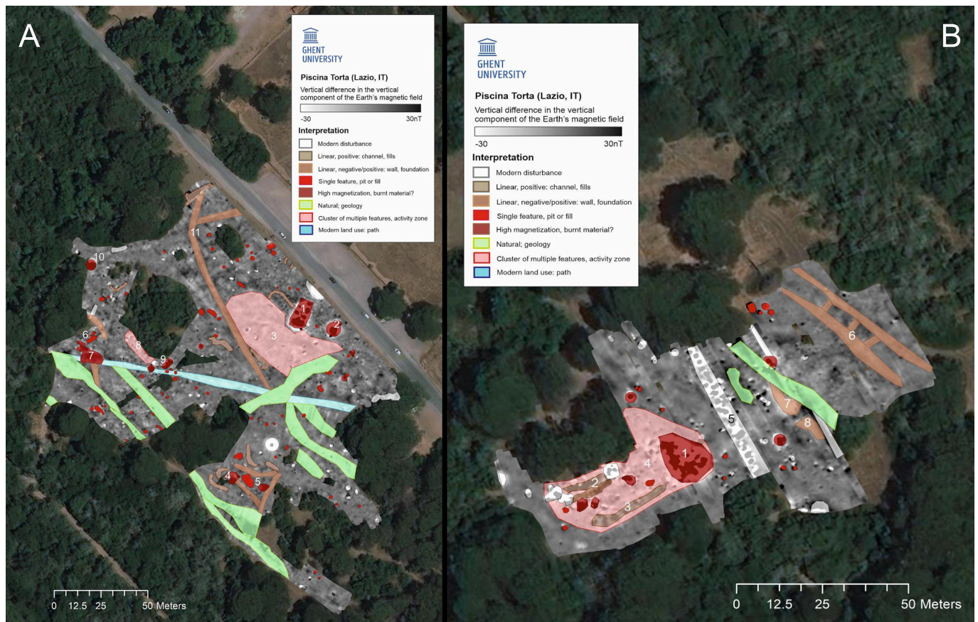
Fig. 9. Interpretation of the magnetic gradiometry data. A, area I. B, Area II. Numbered features are discussed in the text.
