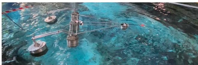
Fig. 5. Aerial photo of WEC with mooring in the wave basin.
