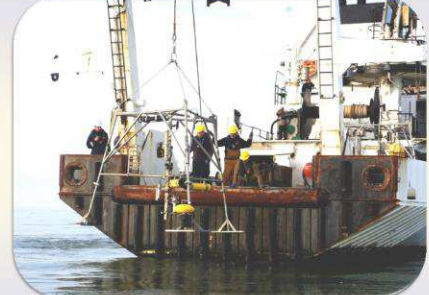
SPM concentration (OBS ADP), Fluid mud layer (ADV altimetry), CTD, LISST, current velocity (ADV, ADP), turbulence (ADV)
