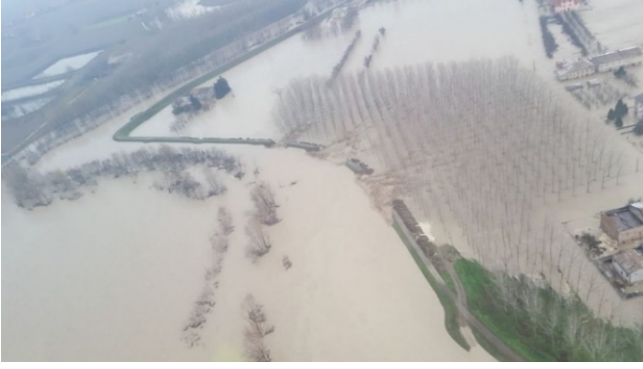
Figure 3. Three simultaneous breaches during the flood event (Reggio Emilia)
