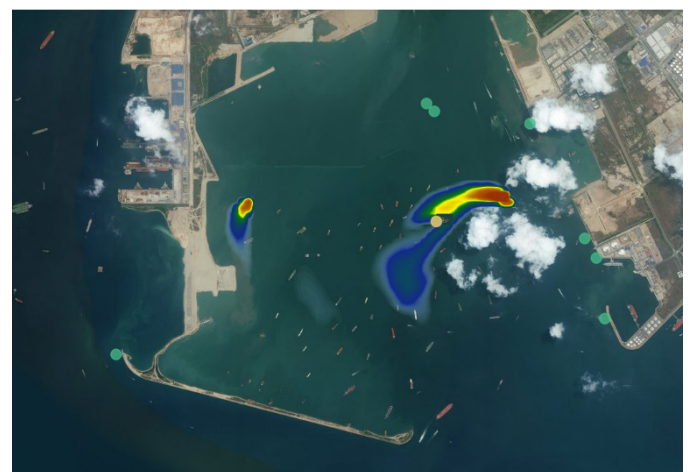
Figure 9. Instantaneous snapshot sediment concentrations due to dredging activities simulated using the coupled near-field far-field model.
