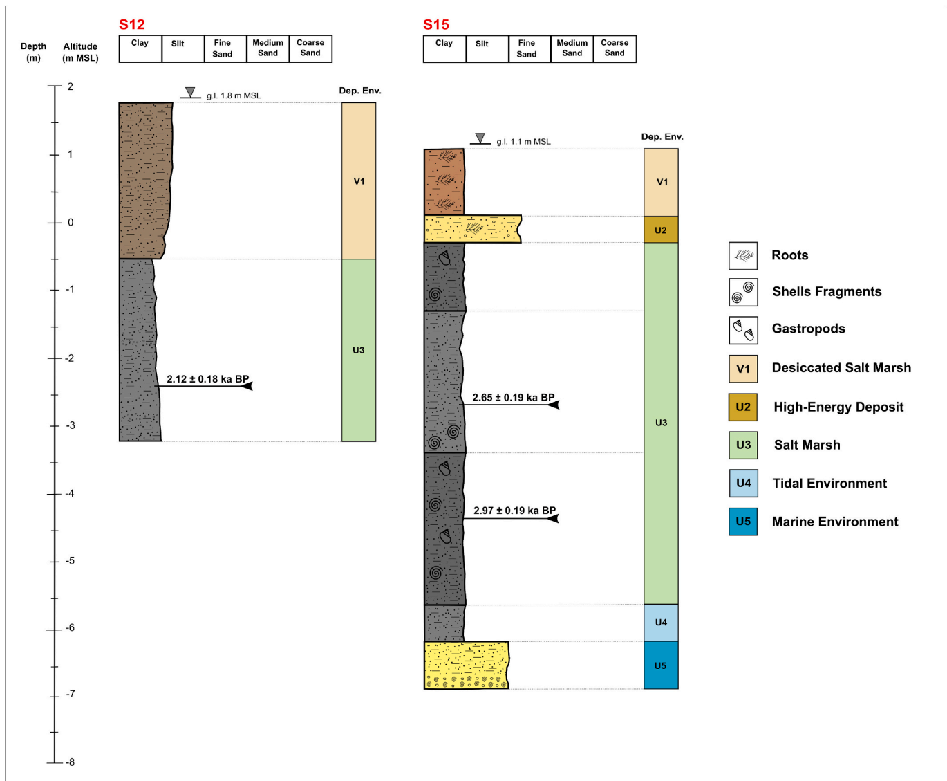
Fig. 6. Schematic stratigraphic logs of the new drillings S12 and S15 carried out in the Southern Bay of Cádiz (for location see Fig. 3).
