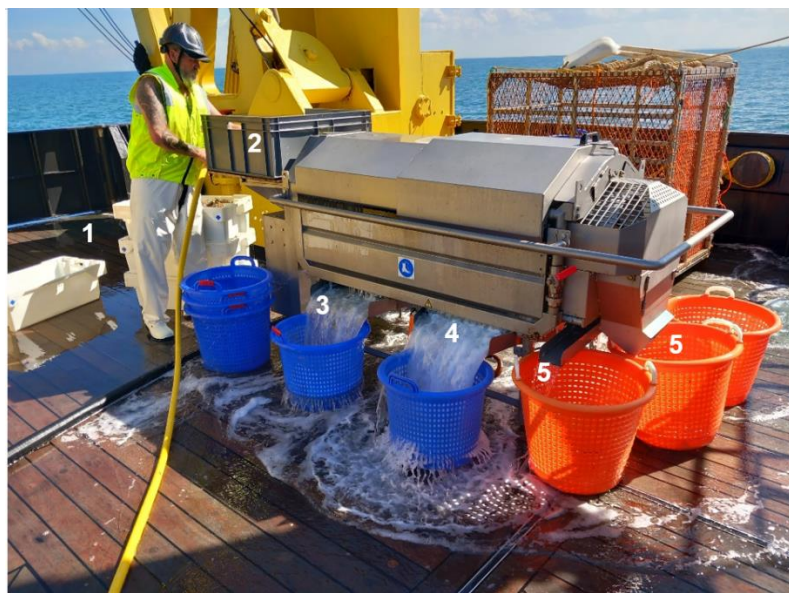
Figure 5-3 Flush sorting machine on board RV Simon Stevin. The collected catch from the pit (1) is emptied into the cistern (2), after which it is divided into three fractions: EPI-S (3), EPI-M(4) and EPI-L(5). These fractions are collected in mutually different baskets. The EPI-S fraction ends up in the blue basket with red handles, the EPI-M fraction in the blue baskets and the EPI-L fraction in the orange baskets. Picture taken on 14/09/2023.
