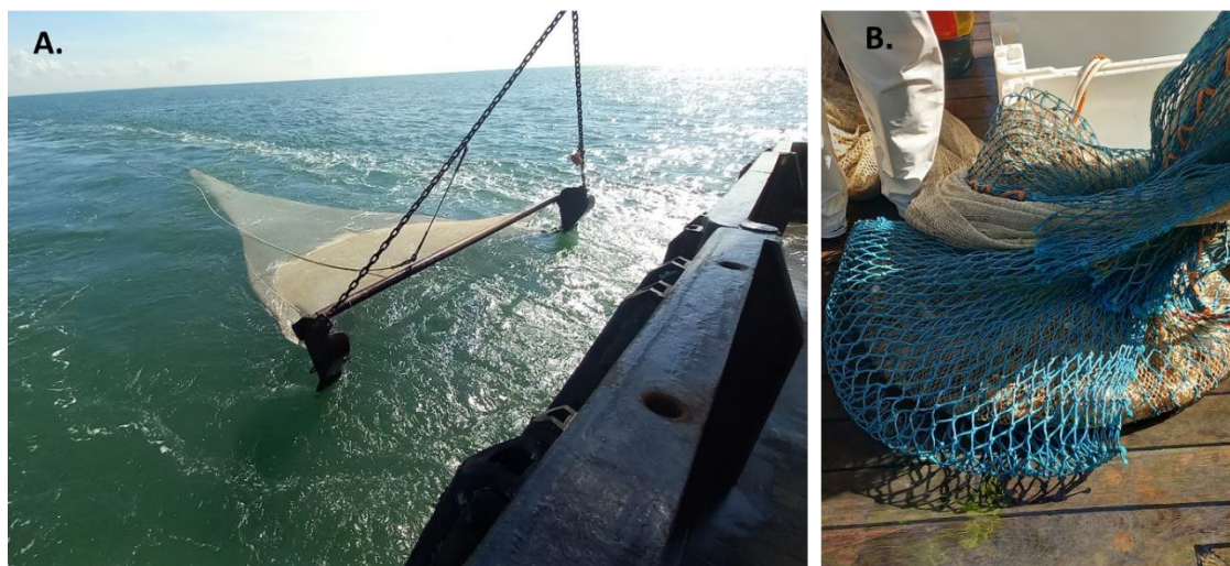
Figure 5-2 [A] The beam trawl which was used during the 2023 DYFS-campaign. The beam trawl has just been put in the water and is ready to be submersed. Picture taken on 14/09/2023 from the stern of RV Simon Stevin. [B] Detailed picture of the pit of the beam trawl. The pit is still filled with the catch of the haul and is ready to be opened. Picture taken on 13/09/2023.
