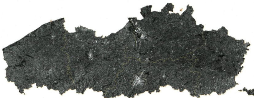
Fig. TAP 3: The SarScape image of Flanders shows the structural characteristics of the landscape which are relevant for atmospheric transport and deposition modelling (aerodynamic surface roughness). SarScape is based on textural features of satellite radar images.
