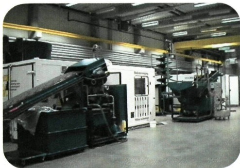
Fig. MIT 3: The PILBO (Pilot for soil washing) is used for solving soil, sludge and solid waste problems. The facility allows to apply sequences of different separation and cleaning techniques to relevant quantities of contaminated samples.
