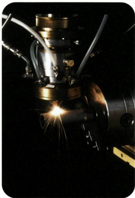
Fig. MAT 1: Lasers can be used to apply wear and corrosion resistant coatings on components with complex geometries. The picture shows a co-axial laser cladding head, which was specifically designed for this purpose.
