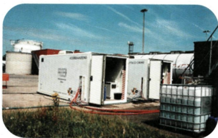
Fig. MIT 6: Pilot test for waste water treatment at the site of a tank cleaning company. The addition of coagulants and flocculants allowed to reduce the amount of suspended solids in the effluent.
