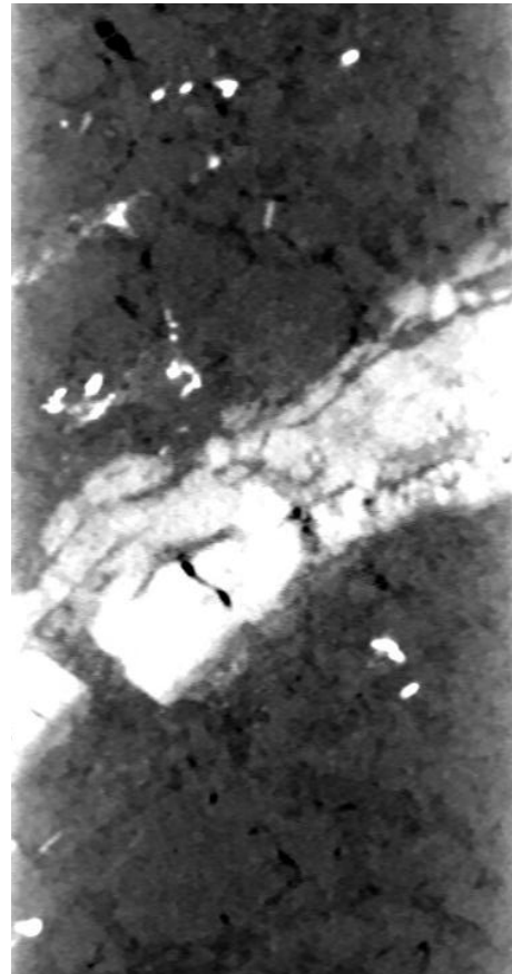
Figure 5. Higher density zone (lighter coloured) and brecciation observed in a sample taken in the vicinity of a shear zone
