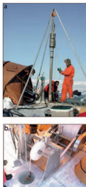
Figure 2. The GreenICE sediment cores were retrieved by a 2 m long gravity corer (200 kg core head) suspended from a tripod and handled by a custom made hydraulic winch through a hole drilled in the sea ice. Photos by Yngve Kristoffersen (a) and Sibylle Göbell (b).
