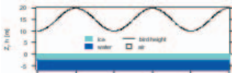
Figure 3. Sketch of model parameters used for synthetic HEM ice thickness assessment. System height varies sinusoidally between 10 and 20 m over a 3 m thick ice layer. A total of 1000 data points is calculated.
