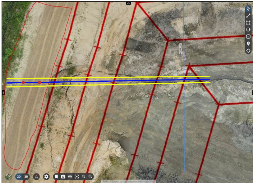
Figure 2. Extrapolation from the observed fault to the identified drilling locations
