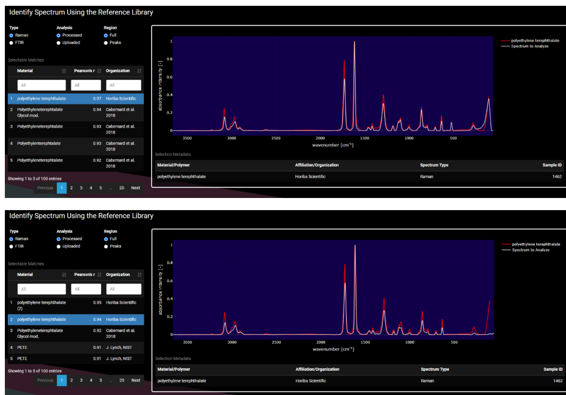
Figure A4.2. Raman spectroscopy characterization of aged polyethylene terephthalate microplastics (MPs, top) and nanoplastic particles (NPs, bottom) with reference spectra from Open Specy reference library. The displayed white spectra correspond to the Raman signals of chemically aged PET particles, while the red spectrum represents the reference material of PET as indexed in the database. The table on the left lists the top spectral matches with a similarity index, indicating a high spectral match score of 0.97 and 0.94 between the aged PET MPs and NPs samples and the reference PET spectrum, respectively. Spectral data are measured in wavenumbers (cm -1 ), highlighting the unique vibrational fingerprints indicative of PET's molecular structure.
