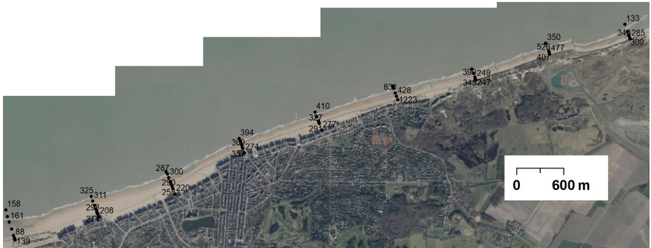
Figure 4 – D50 ( \mu\text{m} ) of sediment collected on the beach along the project site in winter 2021
