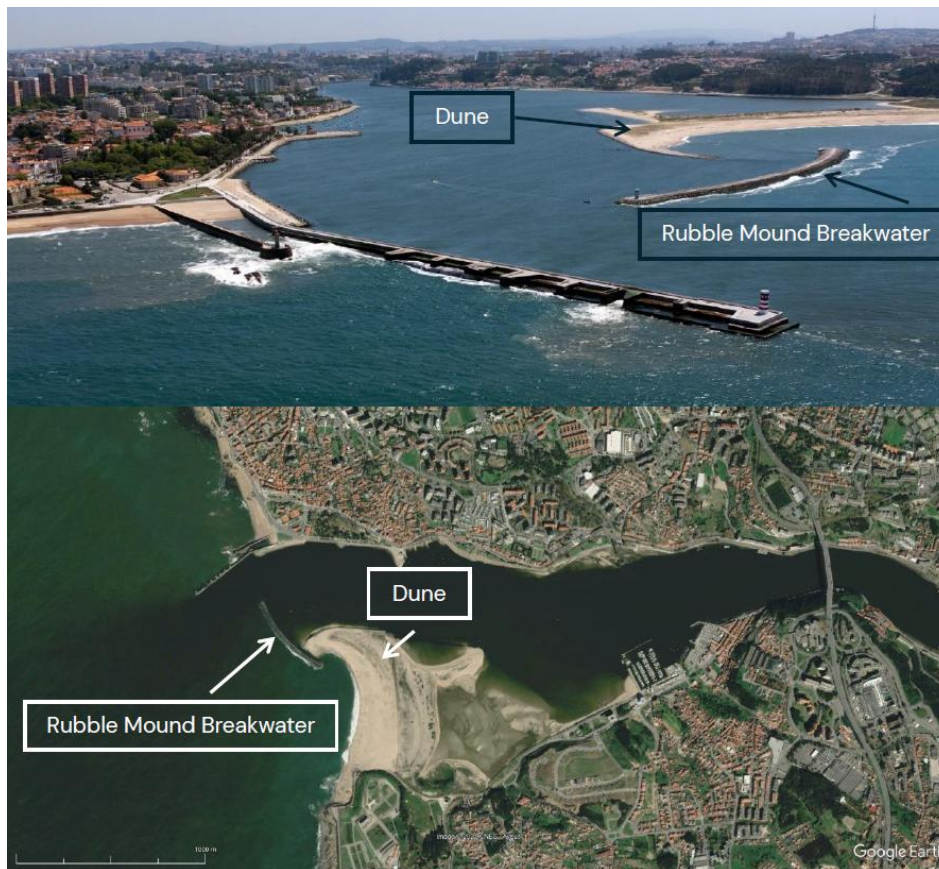
Figure 2: Douro Estuary Sandspit (PT) Demonstrator, a rubble mound breakwater in front of a Dune
