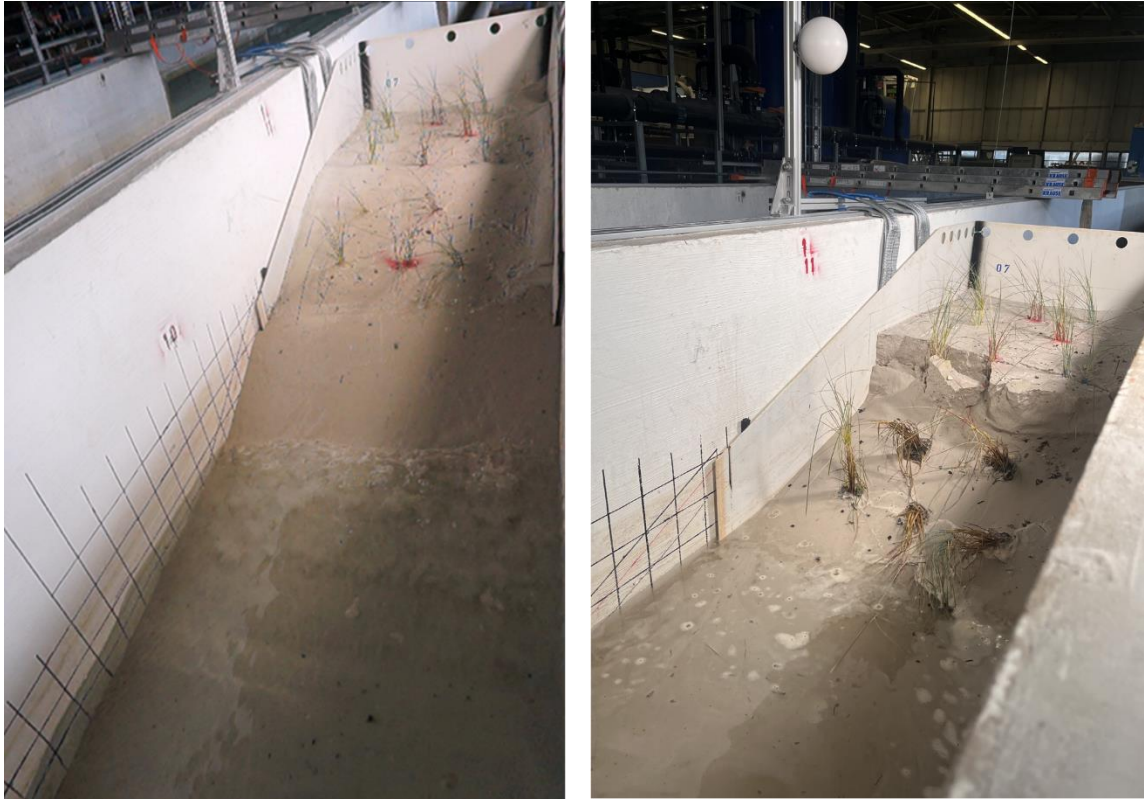
Figure 26: Dune crate containing plants from the burial treatment before (left) and during the wave flume tests (right).
