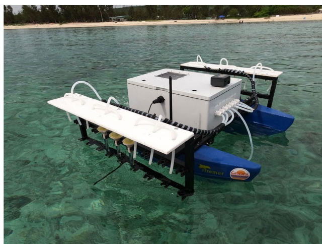
FIGURE 2 | One of the two in-house built Unmanned Surface Vehicles (USVs) during deployment. The pump and associated equipment are contained within the metal box sitting atop the catamaran base, while the yellow capsules below the white plates are the housing units containing the filter membranes. The housings have tube extenders that reach into the surface of the water to enable filtration. The catamaran base possesses two propellers for locomotion (not shown). Photo credit: Mervyn Ravitchandirane.
