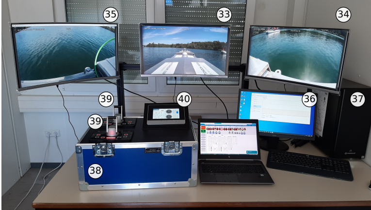
Figure 6.6: Constructed inland SCC streaming video data from the USV sailing on the Rotselaar lake (see Section 6.5.1), part numbers refer to Table A.1.
