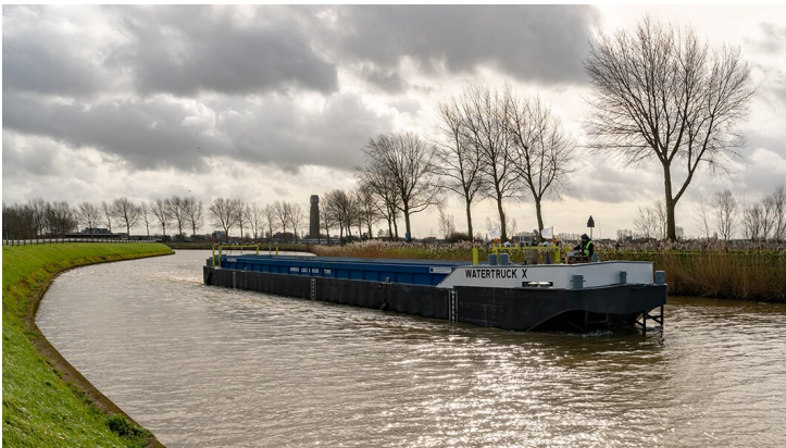
Figure 2.2: A self-propelled watertruck barge sailing on a river [7]. The skipper and steering interface can be seen at the bow of the vessel.
