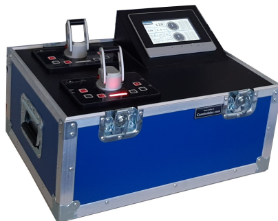
Figure 6.5: The inland SCC motion control subsystem: two azimuth controllers on the left and a touch screen on the right.
