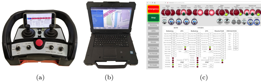
Figure 6.2: The previous line-of-sight shore side control components (summer 2019): (a) wearable remote controller with web-interface, (b) the rugged computer (R-PC) running MOOS-IvP, and (c) an additional laptop monitoring the PLC web-interface.
