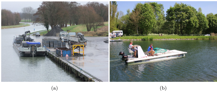
Figure 2.14: The pallet shuttle barges: (a) a real-size Zulu handling cargo at a quay [29], (b) the scale model named Maverick.
