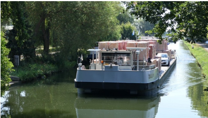
Figure 2.3: A pallet shuttle barge (Zulu 01) sailing on a canal [30]. The skipper and steering cabin can be seen at the bow of the vessel.
