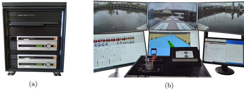
Figure 6.9: Current H2H-extended inland SCC configuration: (a) the combined H2H Engine, and (b) the H2H application running in the inland SCC.
