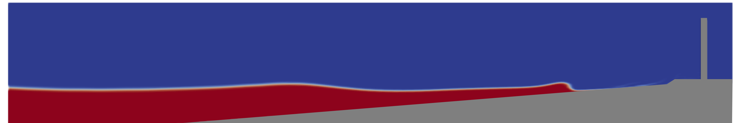
Snapshot of an OpenFOAM result of wave propagation on a sloping beach with a dike and a wall (air: blue, water: red, beach + dike + wall: grey).
