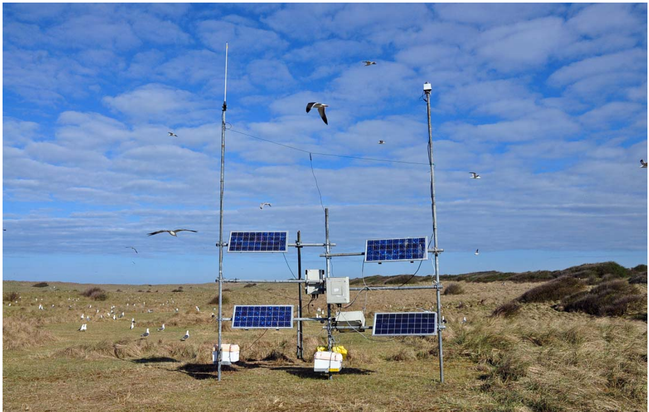
Figure 56. "Houston Control", solar panels and base station set-up in 2010, Kelderhuispolder colony, Texel. The base station has a central position in the colony, and most birds with GPS loggers attached are within 50m in the background and to the left of the base station. A dongle (small object on a string between the two larger poles) provides internet facilities, so that the data could be downloaded remotely (CJ Camphuysen).
